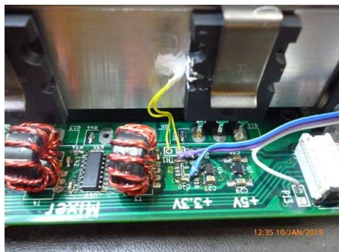
The new local oscillator installation is complete. Inspect the board carefully to insure stray solder is not present and no components have been accidentally moved. The main circuit board needs to be re-installed in the box.
