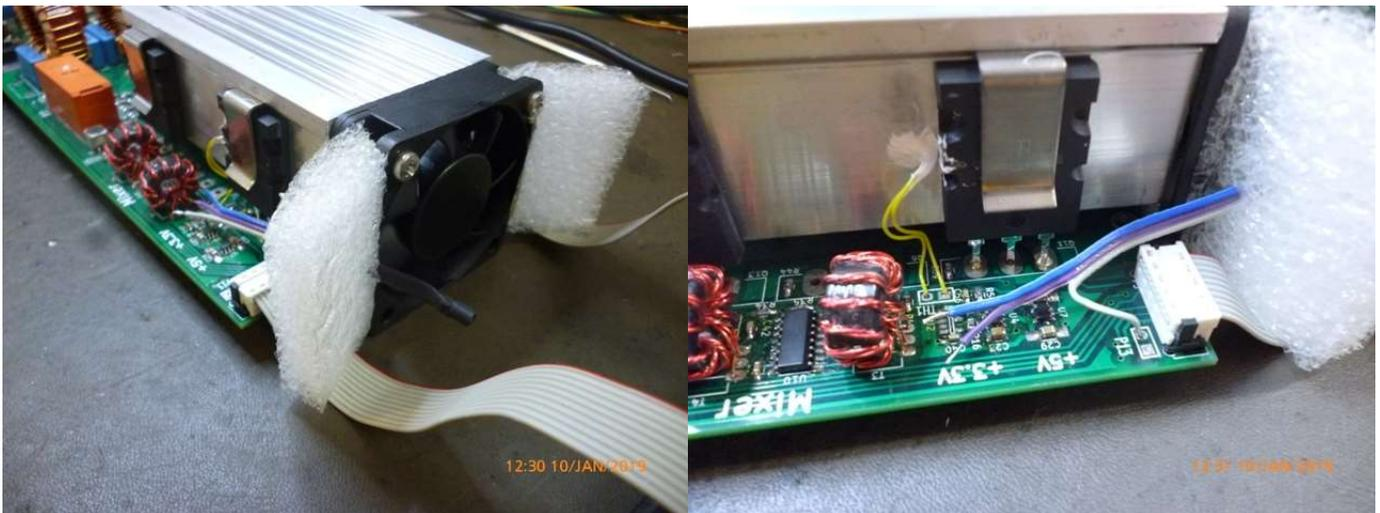
Next solder the purple wire, which is the middle wire of the three. It goes to one end of C36, the end nearest the coil. Note that C36 is not actually used in the circuit but it provides a larger connection point for the wire than just the solder pad alone. Finally solder the blue wire to one end of C40, the end nearest to R16. It should look like this:
