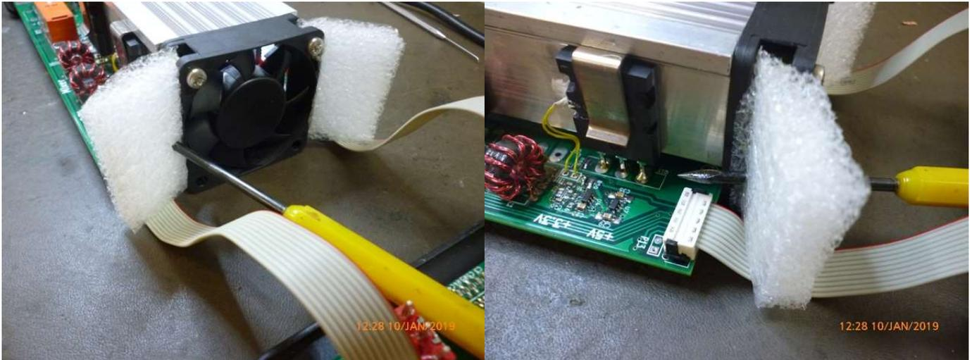
Feed the new oscillator assembly through the hole from back to front. Now solder the white wire to P13, round hole. The round hole is furthest from the board edge. The P13 square hole is connected to 12 Volts, which will destroy the oscillator, so be careful to use the round hole, which is ground.
