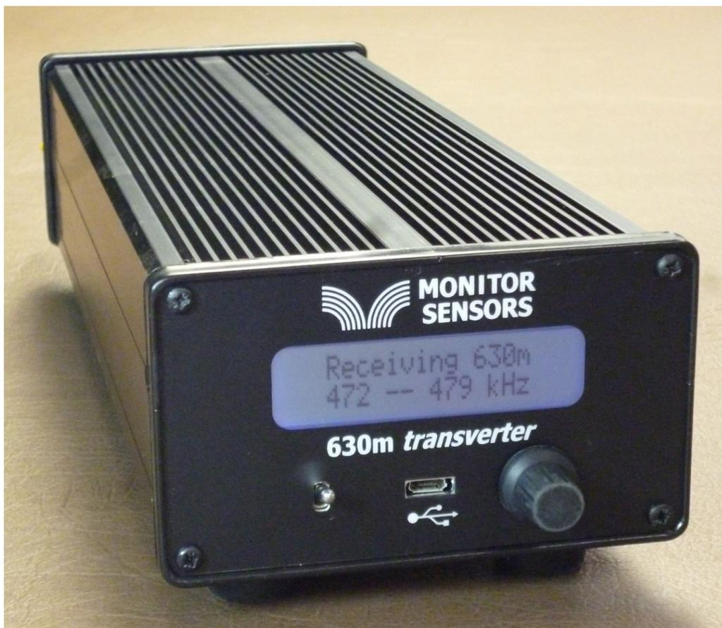
The Monitor Sensors 630m Transverter enables any Amateur Radio Station, equipped with a conventional HF transceiver, immediate, all mode, access to the new 472-479 kHz, 630m band.
